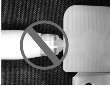
Figure 5: Pipette tip improperly seated into the injection port.
