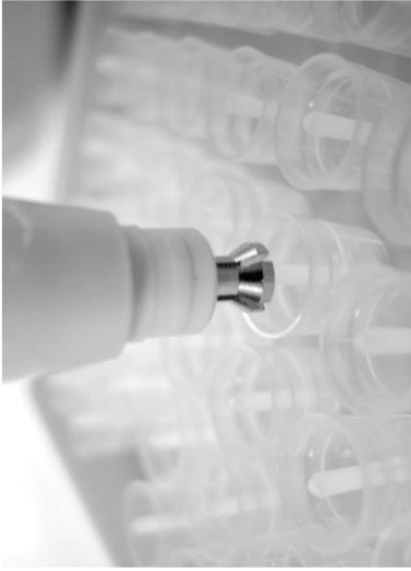
Figure 1: Metal tip in pipette extended to grip the pipette piston.
