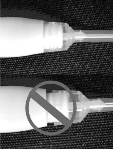
Figure 2: IMPROPERLY vs. PROPERLY seated pipette tip.
