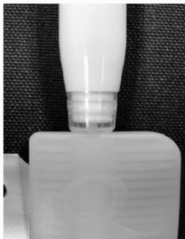
Figure 4: Pipette tip properly seated into the injection port.
