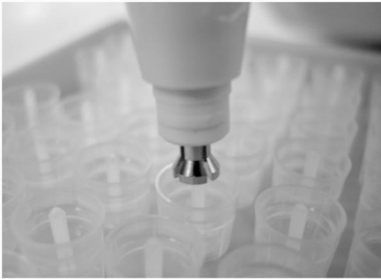
Figure 1: Metal tip in pipette extended to grip the pipette piston.
